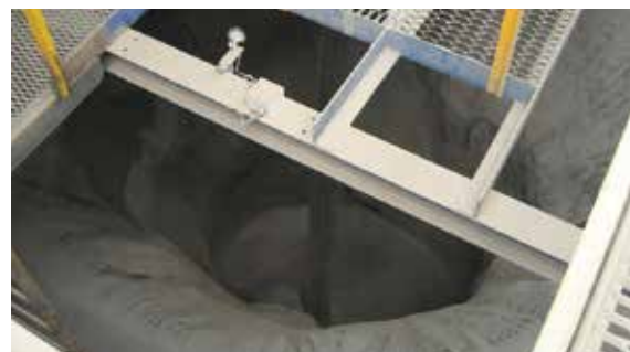
Rathole: The centre portion of the bin empties first in the form of a funnel.
