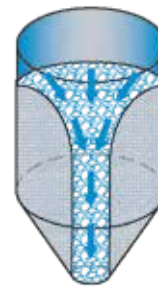
Funnel Flow: The flowing material (blue) is forming a funnel, while the rest (grey) is sticking to the walls of the bin.
