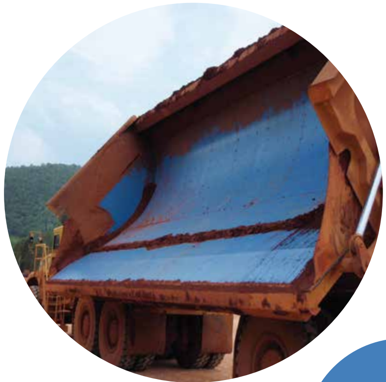
Side tipper truck tray after installation of Matrox
