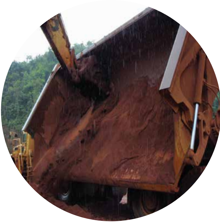
Side tipper truck tray before installation of Matrox lining
