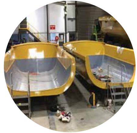
Matrox Off-road truck lining
