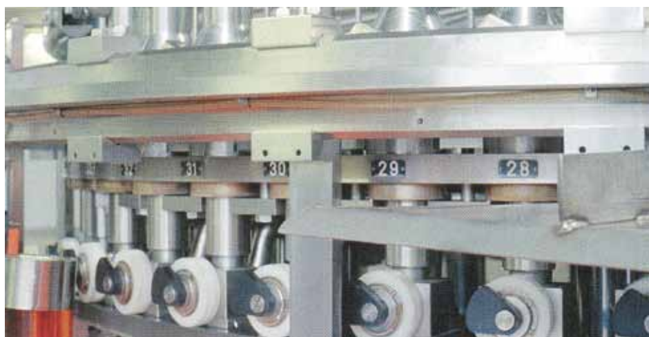
ERTALYTE® camrollers on can filling machine
